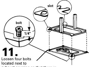
exhaust opening so that there is approximately 1/4 inch space between bolt head and canopy. Lift canopy and insert bolts into slots in support system frame. Tighten bolts to support system frame and canopy.
